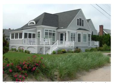
(Saco, ME) Mitigation measures such as bolting vertical surfaces to the foundation and using hurricane-resistant shingles paid off for owners of this home during 2007 Nor-Easter.
