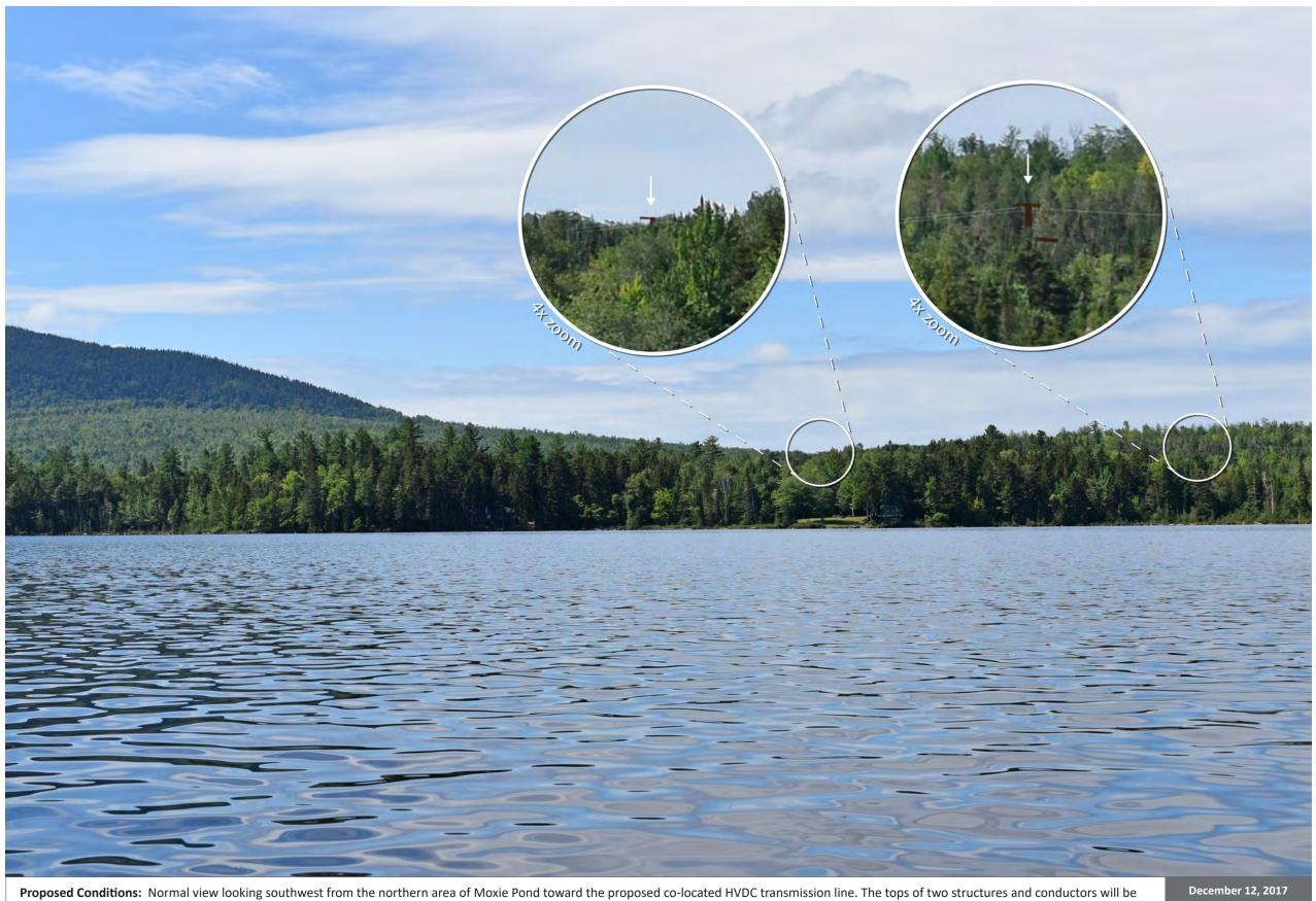
visible from this viewpoint at distances of 2,500 to 2,800 feet . The existing 150' wide corridor clearing will be widened by 75' on the western side to accommodate the new transmission line.
