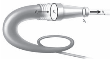
When forced to travel through a smaller space ( S_2 ), water will move at a higher velocity ( V_2 ) Illustration © Kelly Finan, all rights reserved
