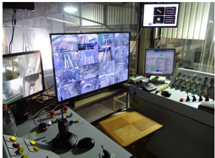
4. Sawyer Booth controls laser scanning and robotics.
