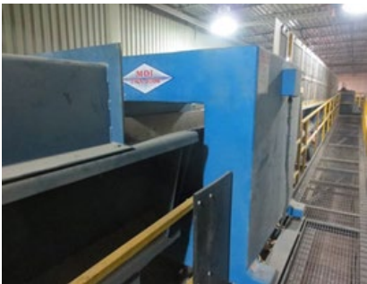
3. Metal detector scans for nails, wire, and other metals.
