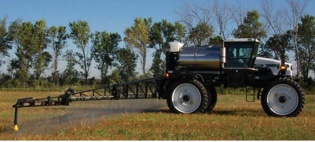
Fine drops are generated from the best drift-reducing nozzles and may stay suspended in an inversion and drift laterally onto sensitive sites.
