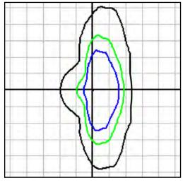
The plot is in units of mounting height of 25'.
