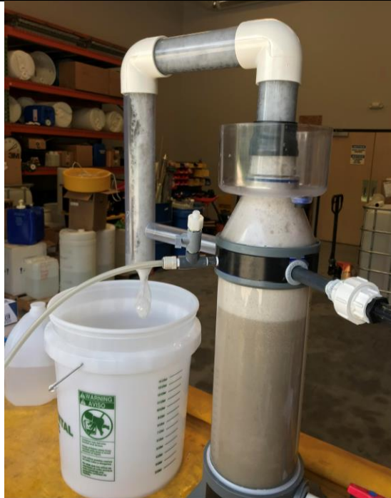
Figure 2. Bench foam fractionation unit used for testing
