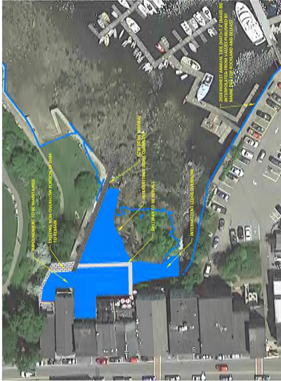
Figure 51. Schematic drawing of full spillway reconstruction with Denil fish passage along a conceptual alignment over the ledge outcrop. Imagery shown represents low tide condition (imagery source: Google Earth).
