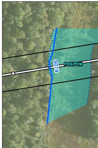
Proposed generator lead crossing of stream S074. From Figure 29 Delineated Natural Resource Map by Stantec Consulting.
