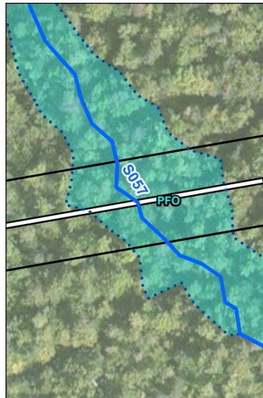
Proposed generator lead crossing of stream S057. From Figure 25 Delineated Natural Resource Map by Stantec Consulting.
