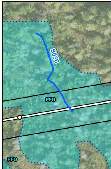
Proposed generator lead crossing of stream S056. From Figure 24 Delineated Natural Resource Map by Stantec Consulting.
