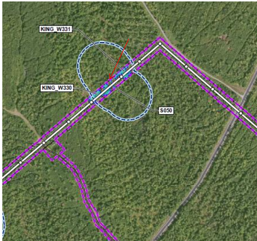
Proposed generator lead crossing of stream S050. From Figure 21 Delineated Natural Resource Map by Stantec Consulting.
