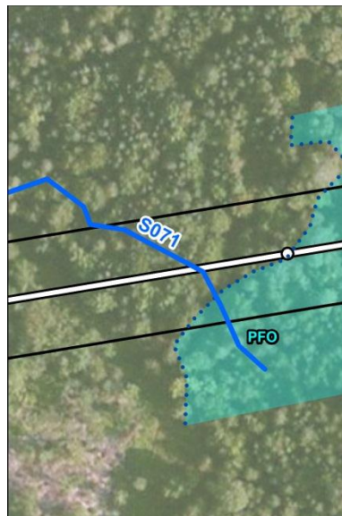
Proposed generator lead crossing of stream S071. From Figure 28 Delineated Natural Resource Map by Stantec Consulting.
