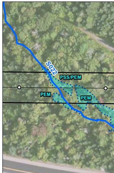
Proposed aboveground collector line crossing of stream S022. From Figure 10, Delineated Natural Resource Map by Stantec Consulting.
