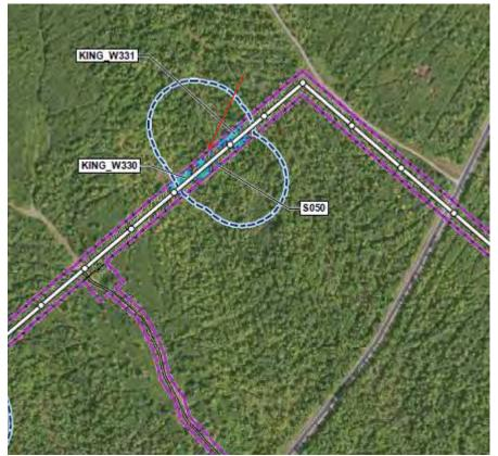
Proposed generator lead crossing of stream S050. From Figure 21 Delineated Natural Resource Map by Stantec Consulting.
