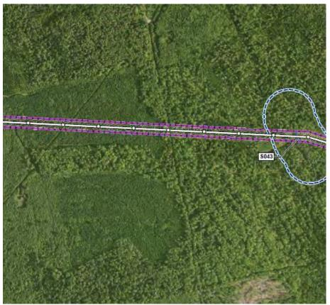
Proposed generator lead crossing of stream S043. From Figure 19, Delineated Natural Resource Map by Stantec Consulting.
