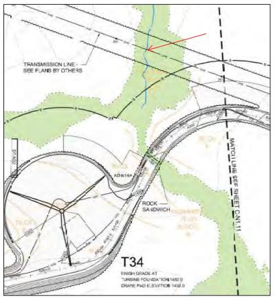
Proposed aboveground collector line crossing of stream S036.
