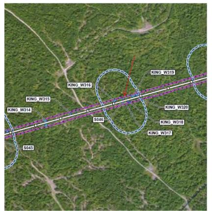
Proposed generator lead crossing of stream S046. From Figure 20, Delineated Natural Resource Map by Stantec Consulting.
