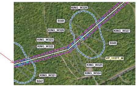
Proposed generator lead crossing of stream S047. From Figure 21 Delineated Natural Resource Map by Stantec Consulting.
