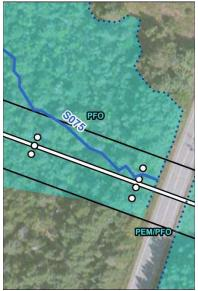
Proposed generator lead crossing of stream S075. From Figure 30 Delineated Natural Resource Map by Stantec Consulting. Intermittent Stream Summary Table
