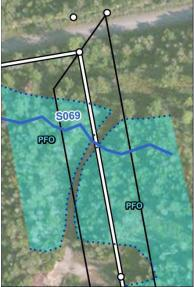
Proposed generator lead crossing of stream S069. Note no proposed impact to wetland ABB\_W384. From Figures 27 & 28 Delineated Natural Resource Map by Stantec Consulting.
