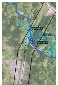
Proposed aboveground collector line crossing of stream S027. Note wetland MAY\_W176 is located northwest along the existing access road and is not impacted by the proposed project. From Figure 11, Delineated Natural Resource Map by Stantec Consulting.
