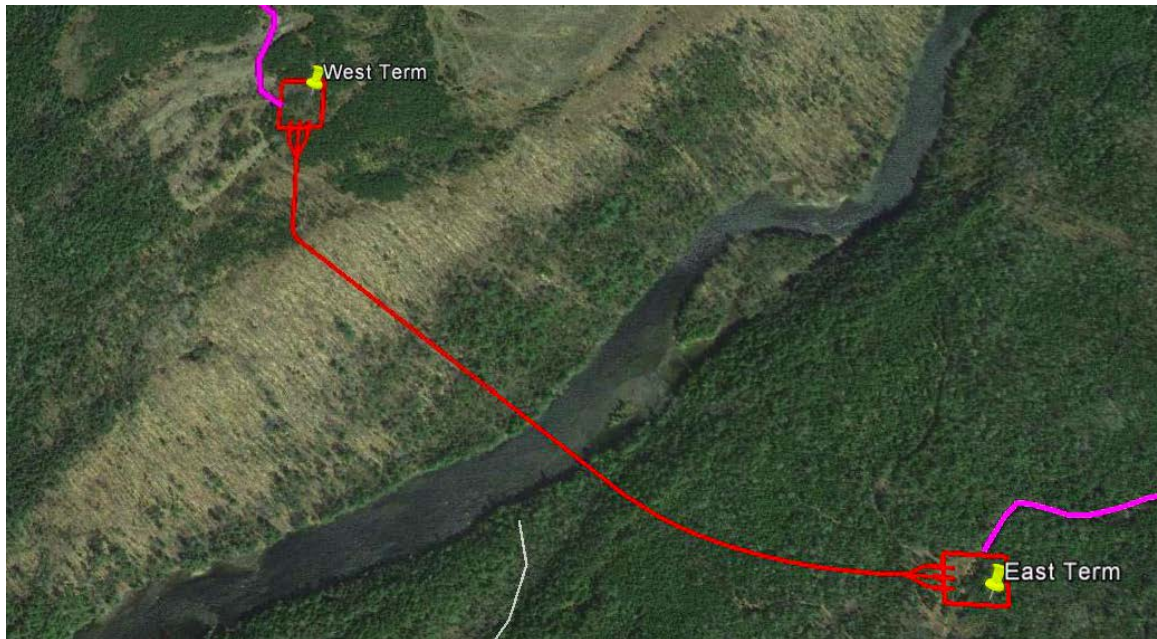
NECEC \pm 320 -kV HVDC Underground Transmission Line - Kennebec River Crossing
