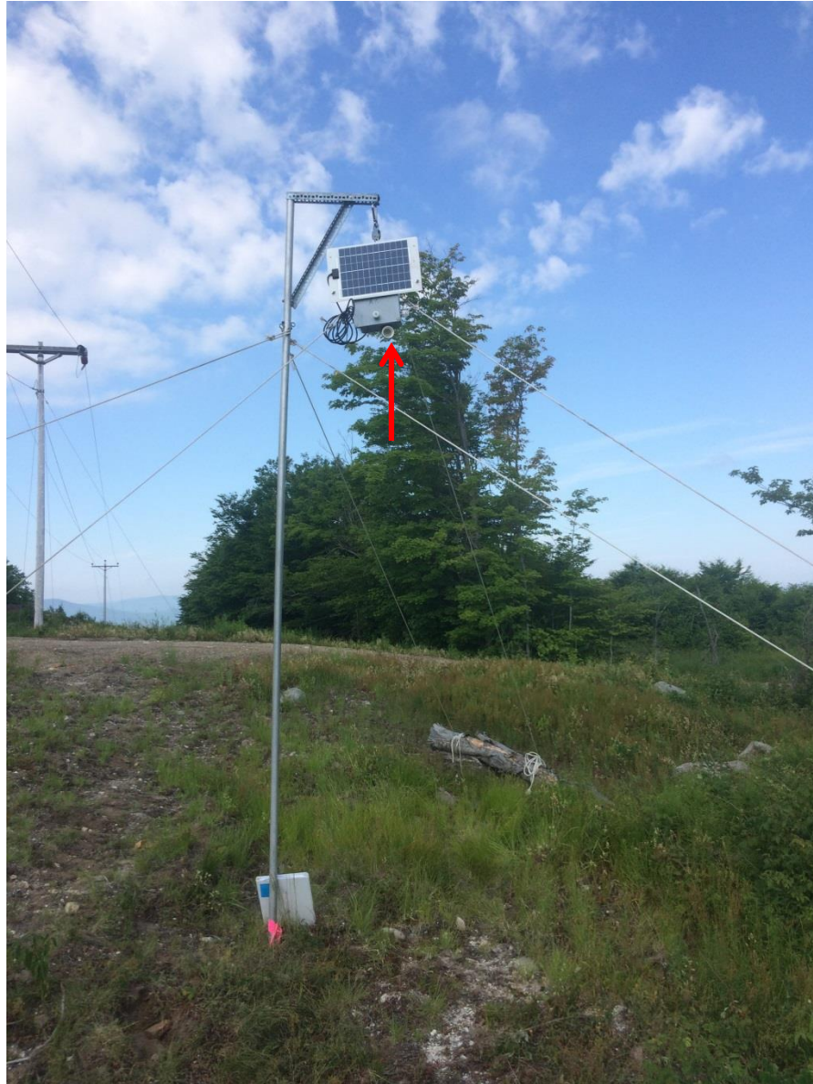
Photo 2: Anabat SD1 detector in weather proof casing deployed in the transmission corridor at the Horseshoe Valley Wind Project for northern long-eared bat surveys in June 2016. The arrow indicates the 90-degree angle PVC-elbow attached to the weather proof casing over the detector, protecting to microphone from adverse weather conditions and funneling sound from the potential flight corridor to the microphone.
