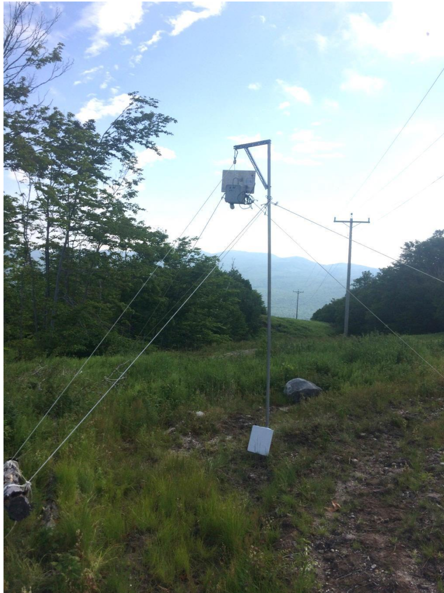
Photo 1: Anabat SD1 detector in weather proof casing deployed in the transmission corridor at the Horseshoe Valley Wind Project for northern long-eared bat surveys in June 2016. The detector is located approximately 3 m above vegetation height, oriented horizontally to the ground, and facing 67°. A 3-ring binder is placed at the bottom of the detector for scale.
