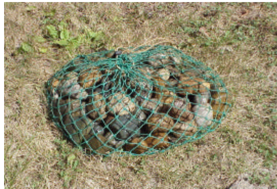
Fig. 7. Rock-filled riffle bag for sampling streams less than 10 cm deep
