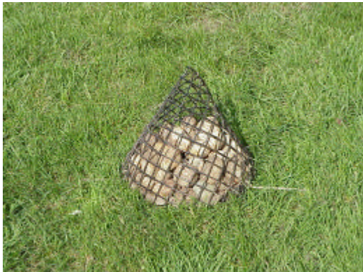
Figs. 8-9. Remote-retrievable rock-filled cone and retrieval funnel for sampling non-wadeable rivers
