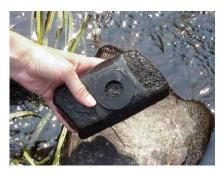
Figure 8. Wrapping sampling device around cobble
