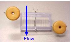
Figure 5. Durasampler® 40-slide Periphytometer
