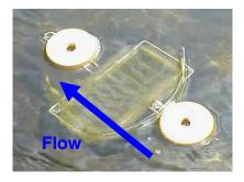
Figure 6. Direction of flow for Wildco® Periphytometer
