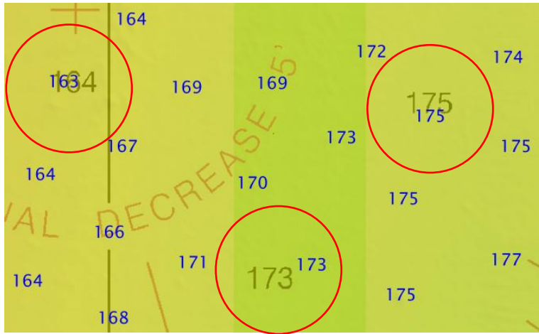
Figure 8 In flat regions charted soundings and gridded data agree very well, generally within a foot, throughout survey area.
