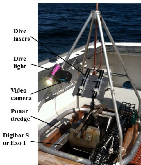
Figure 2. MCMC grab sampling platform.
