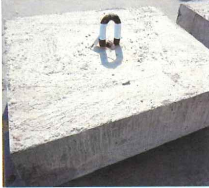
Concrete Moorings Length: 36-inches Width: 18-inches Height: 12-inches Weight: ~2000 pounds
