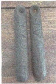
Counter weight - for depth control line ~10 lbs
