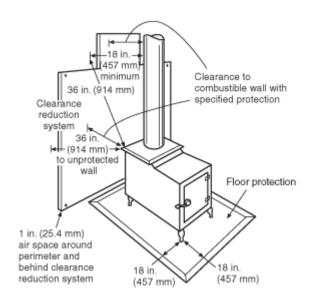
FIGURE 12.6.2.1(b) Distance to Combustible Wall/Floor.
