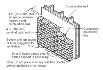
FIGURE 12.6.2.1(c) Masonry Clearance Reduction System.
