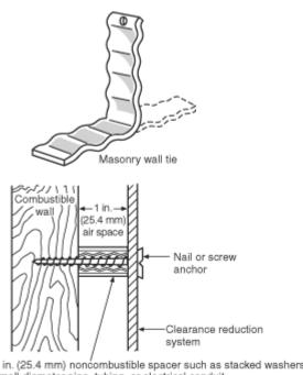
1 in. (25.4 mm) noncombustible spacer such as stacked washers, small-diameter pipe, tubing, or electrical conduit
