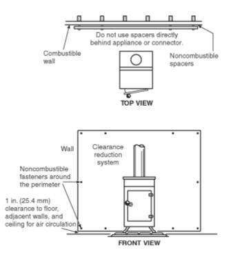
FIGURE 12.6.2.1(a) Clearance Reduction System — Fastener Location.
